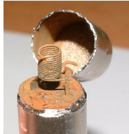
Fig 6.2.1 Internal Corrosive Damage Caused by Incorrect use in Aggressive Humid Environments
